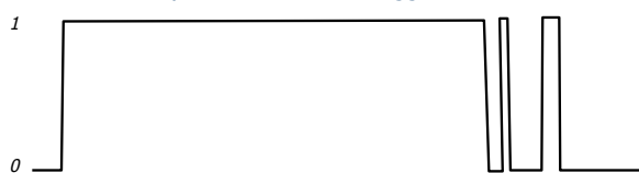
Digital Value Read by PIC with Schmitt Trigger:
